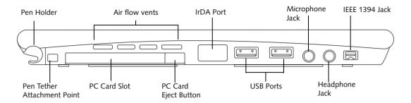
Figure 1-4 Stylistic ST4000 Series Tablet PC Features (Top View)
